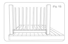
Cut the top rail following the same procedure that you used in steps 3 and 4 for the bottom rail.
