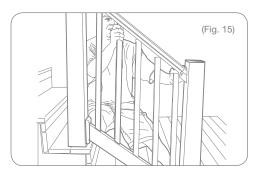
To allow for baluster expansion, raise the top rail approximately ½. Pre-drill the holes for the mounting brackets to avoid stripping the stainless steel screws (Fig. 16).
