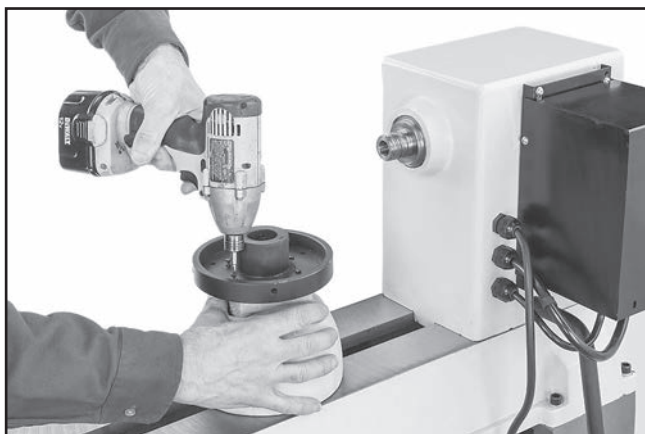
Figure 39. Typical attachment of faceplate to workpiece.
