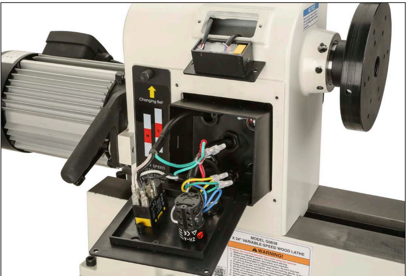
Figure 58. RPM readout display board and control panel wiring.
