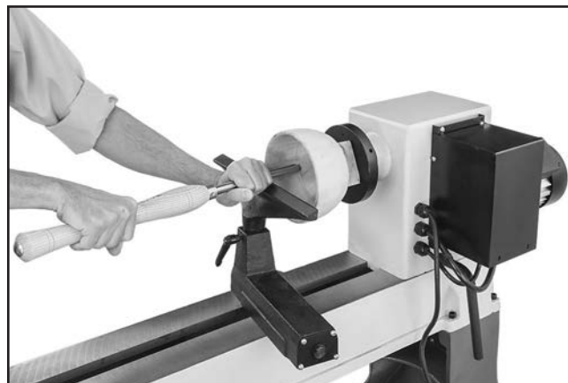
Figure 38. Typical faceplate turning operation.
