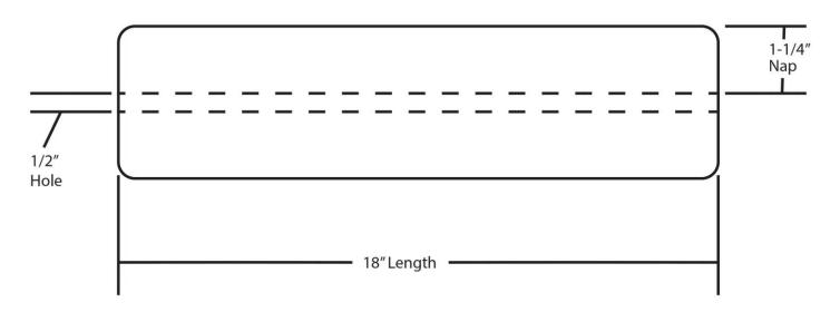
\*For use with adjustable frame roller with a 18" capacity.
