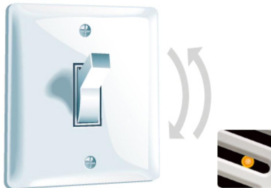
Cycle on/off switch to operate at full speed mode, & LED indicator light is AMBER
