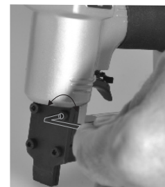
Fig. 4 - Removing the Nosepiece: Unscrew the 4 nosepiece screws to release the nosepiece.
