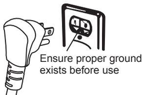
Do not use an adapter plug. Disconnecting of the power cord places undue strain on the adapter and leads to eventual failure of the adapter ground terminal.
