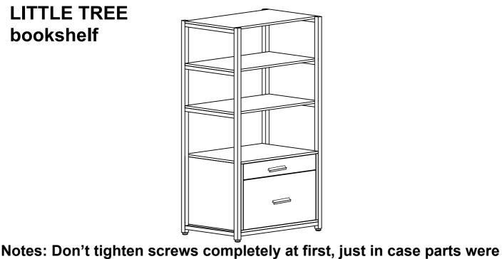
assembled wrong and need disassemble. Tighten screws at last when all parts are put together
