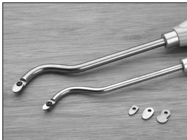
Figure 48. Swan neck hollowing tools.
