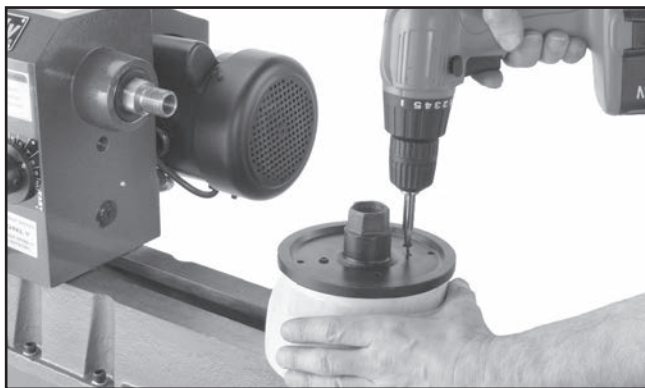
Figure 38. Typical attachment of faceplate to workpiece.
