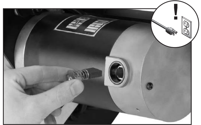
Figure 57. Removing brush from motor.
