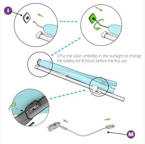
4.You can use the screw to get the battery out of the holder, then charge it with USB wire.
