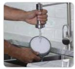
Clean and rinse filter regularly to maintain performance (dry for 24 hours before reinserting)
