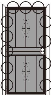
5. Open the door and remove the two pre-hang brackets. Close door, and drill through the remaining holes in the Z-bar with a 5/32" drill bit, and fasten with Phillips head screws provided while keeping a consistent reveal between the door frame and supporting Z-bar.
