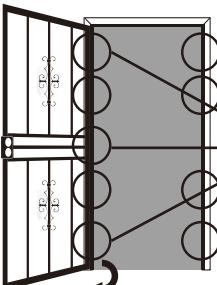
Utilize the pre-drilled concealed screw holes on the inside portion of the hinge side and the lock side of Z-bar for added tamper resistance.
