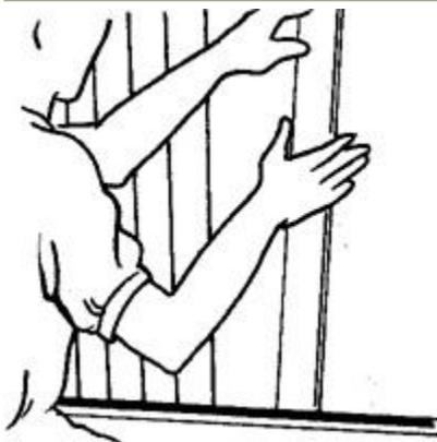
Add new pieces of wainscot by pushing the grooved edge onto the tongue of piece already applied. (See Figure 2.)
