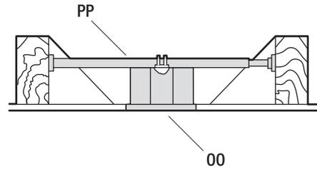
To hang your fan where there is an existing fixture but no ceiling joist, you may need an installation hanger bar (PP) (not included) as shown above.
