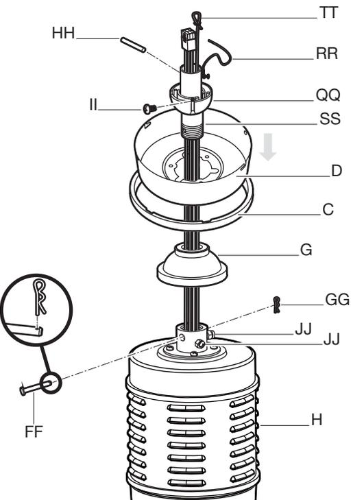
is in the correct position, the setscrew (II) is tightened and wires are not twisted.
