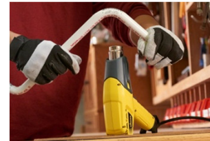
Bending Pipes / Plastic
