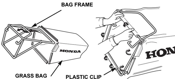
Lift the rear discharge guard, remove the mulching plug, and install the grass bag.
