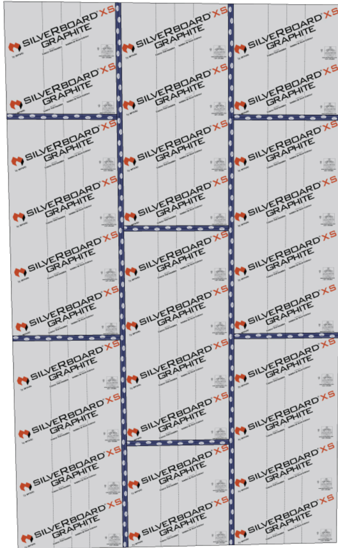
Taping pattern for vertical board orientation
