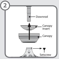
Remove the downrod by unscrewing the bottom set screw. Unscrew the downrod. Remove the canopy and canopy insert. Reinstall the downrod according to the fan manual.
