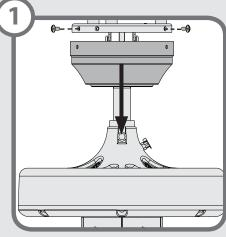
Remove the three canopy screws. Lower the canopy and the canopy insert. With wiring exposed, it may be helpful to note existing wire connections or take a digital photo for reference. Remove the wire connectors that connect the wires from the outlet box to the fan. Unhook the fan from the ceiling.
