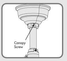
If your fan is already installed and the canopy is held by two screws near the downrod as shown, follow the **TYPE-B ASSEMBLY INSTRUCTIONS** on page 4.
