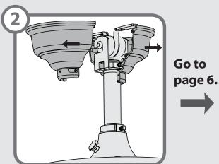
Remove the two canopy halves. With wiring exposed, it may be helpful to note existing wire connections or take a digital photo for reference. Remove the wire connectors that connect the wires from the outlet box to the fan, leaving the grounding wire connected.
