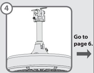
Reinstall the fan according to the installation manual included with the fan, but do not install the ceiling plate, canopy, or canopy insert. Rewire the grounding wire according to the fan manual.
