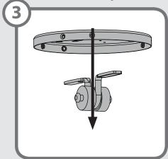
Remove the u-bracket and the ceiling plate from the ceiling.
