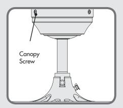
If your fan is already installed and the canopy is held by three screws near the ceiling as shown, follow **TYPE-C ASSEMBLY INSTRUCTIONS** on page 5.
