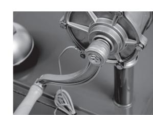
Attach the pump handle (S) to the oil pump. Please must be in correct postion before turning to aviod to demage thread
