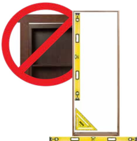
Move lower jamb out half pop distance.
