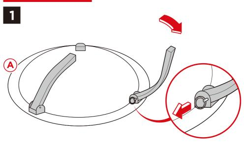
Flip the part A bowl upside down. Pull out the pin on a leg, flip out the leg, then release the pin to lock the leg in place. Repeat on the remaining legs.
