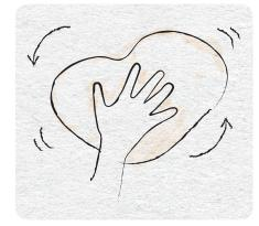
For solvent based adhesive, clean up surface with mineral spiritsdampened rag (do not use lacquer <u>thinner</u>). For low VOC adhesive, wipe off all excess adhesive on the surface with water dampened rag.
