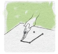
Put the first panel in place and bring to adjacent wall in the corner allowing 1/16"space. Make sure it is plumb and both left and right panel edges fall on solid stud backing.
