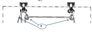
b) Tie one end of the pull cord to the left front bar of the awning, thread
