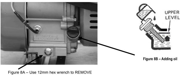
Figure 8A – Use 12mm hex wrench to REMOVE bolt and drain oil
