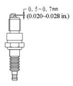
Figure 9 Measuring the spark plug gap
