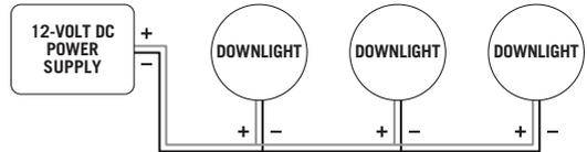
On very large, multi-LED light installations, be aware of possible voltage drop, which only becomes undesirable if you notice the brightness in one area of your lighting is objectionably different than in another area. Do not coil wire; shorter lengths and thicker wire will mean less voltage drop and higher brightness. For an online voltage drop calculator, visit [armacostlighting.com/voltagedrop](http://armacostlighting.com/voltagedrop).
