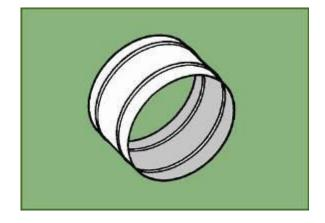
• Sleeves used to connect 2 flex duct pieces together shall be a minimum of 4 inches in length and beaded on each end.
