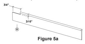
Trim Vinyl Sweep one an a quater inch longer than the Drip Rail, then Notch Vinyl Sweep (H) as shown in **Figure 5a**.
