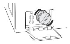
Close the drain pump filter cover.
