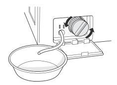
Clean the pump filter and opening.
