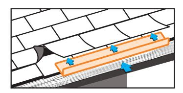
Fasten with 3 hot dipped galvanized roofing nails.
