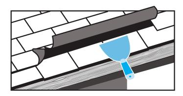
Slide Rain Diverter under shingles as far as it will go, giving it a slight pitch to one side.
