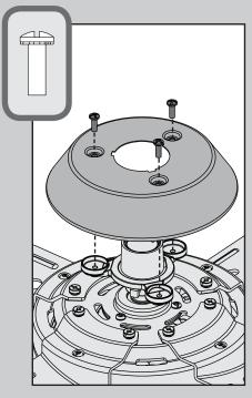
Lower the top housing onto the top of the motor. Install the three top housing screws.
