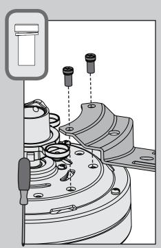
Eightly attach the blade irons to the motor with screws found in the ∑ hardware bag, then securely tighten after both screws are attached.
