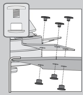
Secure each blade to a blade iron as shown using the blade nuts, found in the hardware bag, and the blade assembly screws, found in the  $\triangle$  hardware bag.
