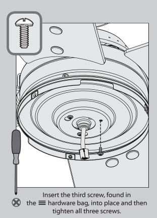
Make sure the upper switch housing is securely attached to the mounting plate. Failure to properly secure all 3 assembly screws could result in the switch housing fixture falling.
