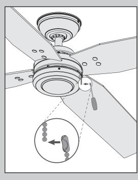
Installing the pull chain pendant - Attach the pull chain pendant to the short chain coming from the switch housing.
