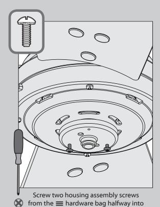
the motor housing. It does not matter
