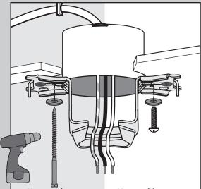
Use wood screws (included) when securing to support structure with approved electrical outlet box. Drill 9/64" pilot holes in support structure to aid in securing ceiling bracket with hardware found in the  $\bigstar$  hardware bag.
