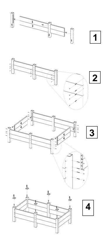
Insert two 1 ½"x5 ½"x 94" rails (part 3) through one 4"x 4"x 19" line post (part 2). Insert ends of 94" rails into two 4"x 4"x19" corner posts (part 1). Slide line
