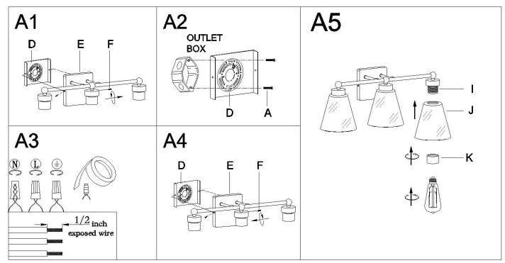
Step A1: Unscrew screws (F) from back plate (E), then set them aside for later installation.
