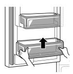
2 To replace the bin, slide it in above the desired support and push down until it snaps into place.
