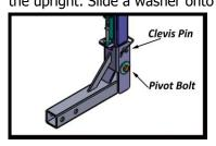
the upright. Slide a washer onto the pivot bolt then slide it through the foot and upright. Put on the second washer on and then secure the nut tightly. Adjust the bike carrier upright to be perpendicular with the foot and insert the Clevis Pin in hole above the lower bolt. Once the Clevis Pin is completely inserted, secure it with the snap pin.
