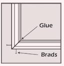
Must moldings are installed with a 90 degree angle joint. Cut 2 pieces of molding with a 45 degree angle each piece and together they make 90-degree angle. Use WPB Cement to glue the ends of the boards. On both sides place fasteners 2" from the end.
