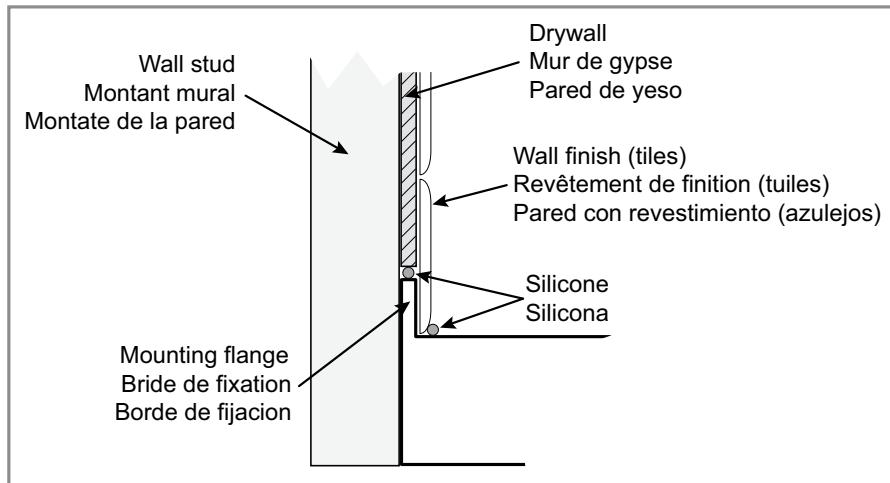
The ceramic wall covering must completely cover the mounting flange. Seal the joint between the unit and the wall covering with a bead of silicone.
