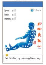
Press "on/off" button when chair power is on, a buzzer beeps once short it. LCD screen display boot screen, after 2-3 seconds it displays the main interface and enter standby mode. Main interface show massage position, method, time, heating current massage status etc., all information will be updated timely when the chair start working.
