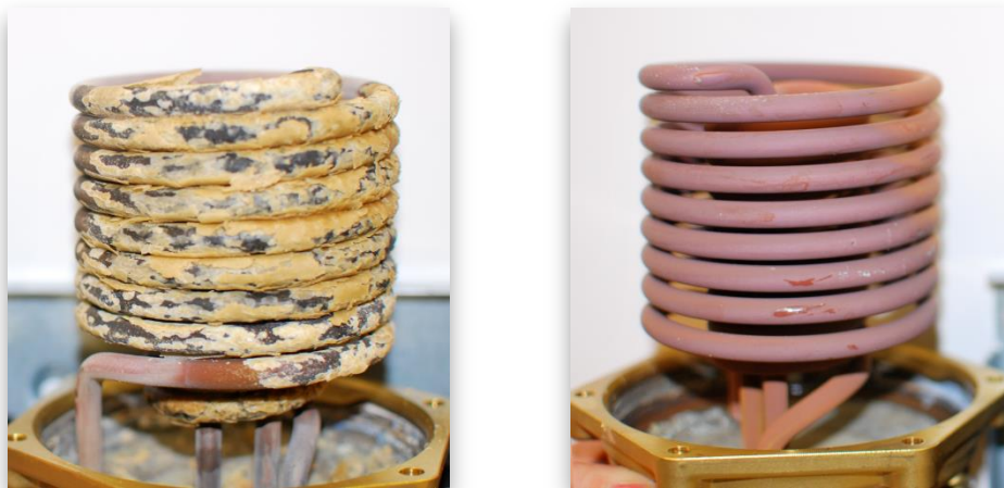
Figure 3. Untreated Element (Left) and Treated Elements (Right)
