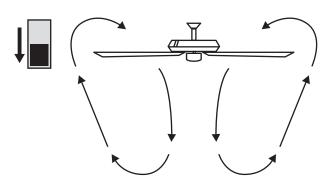
Cool weather - (Clockwise Direction) An upward air flow moves warm air off the ceiling. This allows you to set your heating unit on a cooler setting without affecting your comfort.
