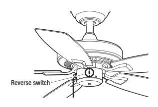
Warm weather - (Counterclockwise Direction) A downward air flow creates a cooling effect. This allows you to set your air conditioner on a warmer setting without affecting your comfort.
