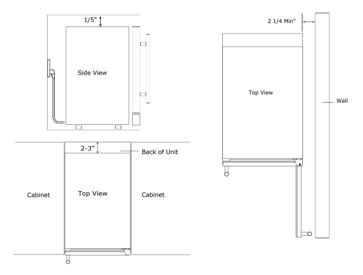
Units have a zero clearance for the door to open 90°, when installed adjacent to cabinets.
