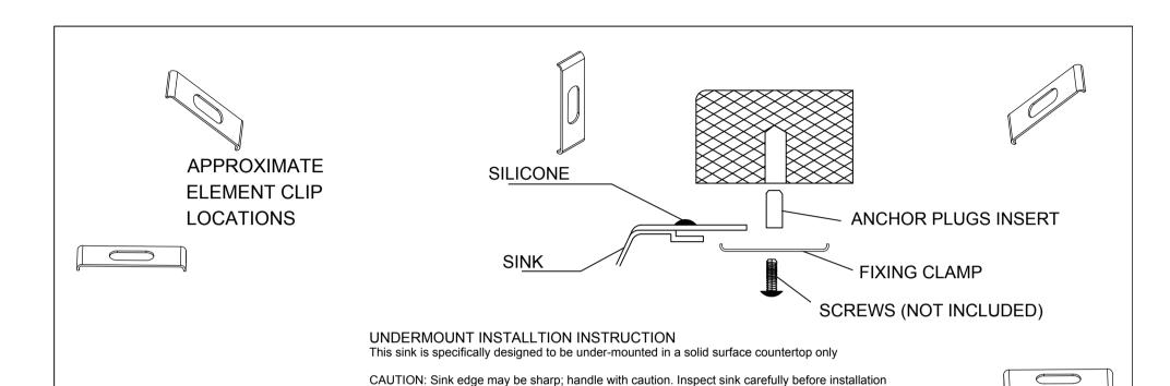
2.Determine placement of clip brackets as indicated by template.Pre-drill holes
