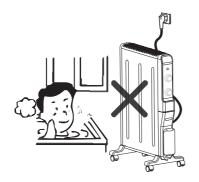
• This heater is not intended for use in bathrooms, laundry rooms, and similar indoor enclosed locations. DO NOT operate it near a bathtub or other water containers.
