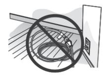
• The use of an extension cord is not recommended, as it may overheat during the operation of the heater.
