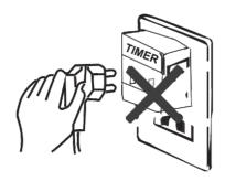
• ATTENTION: in order to avoid any danger caused by an accidental resetting of the safety system, this appliance must not be powered through an external timer.
