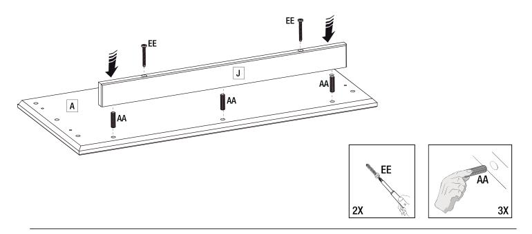
6 Connecting the top panel and placing the floor protection on the side panels
