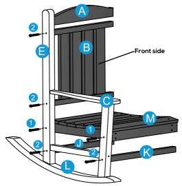
Attach part A Backup plate and part B Chair Backrest to part F Left back leg with 2 pcs of part 2 Bolt. Attach part M Chair seat to part F Left back leg and part D Left front leg with 2 pcs of part 1 Bolt. Attach part K Front rail to part D Left front leg and attach part J Back rail to part F Left back leg with 2 pcs of part 2 Bolt.
