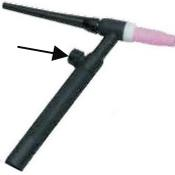
Turn the TIG Torch gas valve clockwise to start the flow of shielding gas. After welding, turn the TIG torch gas valve counter-clockwise to turn off the flow of shielding gas.
