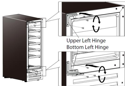
6. Rotate the door 180° so that the top is now the bottom, and install it by attaching the support rod with screws.
