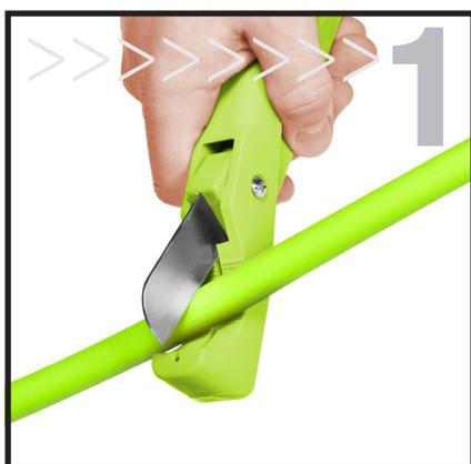
**Measure and cut desired length of hose at 90°.**
