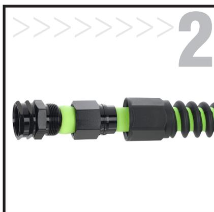
**Slide bend restrictor and fitting nut onto hose. Push the threaded fitting into hose until flush.**
