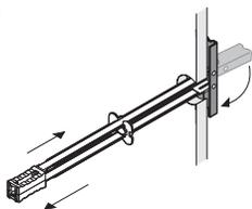
Slide plastic ring along straps until flange of ring is flush against wall.
