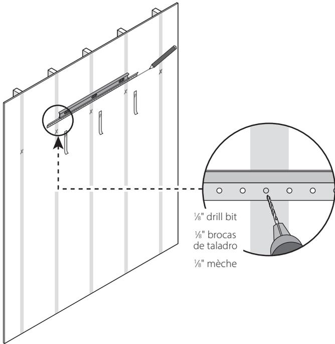
**6 IMPORTANT.** If a vertical will be more than 3" from a stud, you'll need to use a toggle to support that panel. Mark toggle locations next to vertical panel locations. If panel will be less than 3" away, skip to Step 9.
