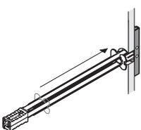
Bend plastic straps back and forth until they snap off, leaving plastic ring in place.
