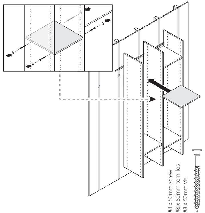
**15** Install cleats under bottom fixed shelves in both towers. Install cleats by using a #8 x50mm screw through the cleat holes into wood studs in the wall. Use a toggle and toggle bolt if no wood studs are available.
