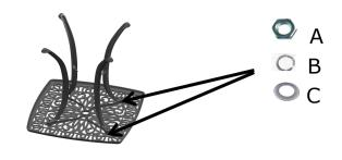
Turn over the table top. Attach the Stud M8(E) into the Nuts(inside table), Then, Attach table Legs((2)) to the Studs on Place all parts on a clean and soft surface the Table Top (1) using Wahers and Nuts (A,B,C).DO NOT over tighten
