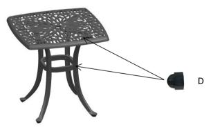
Tighten all Nuts with Wrench.And Turn over the table.Adjust the pre-installed Rubber Pad (L) until the Table is level with the ground ,Tighten all the nuts and cover them with nut caps(D). Your table can use now.
