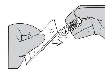
WEAR SAFETY GOGGLES. BLADES ARE EXTREMELY SHARP. HANDLE WITH CARE. WEAR CUT RESISTANT GLOVES TO PROTECT HANDS. DO NOT BEND BLADES. BLADES MAY BREAK IF BENT AND MAY RESULT IN BODILY INJURY. CLOSE OR COVER BLADE WHEN NOT IN USE.
