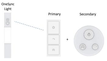
2. Press and hold the CCT button on the secondary remote. While still holding down the CCT button on your secondary remote, press and hold the Dim button on your primary remote. Press and hold both buttons for three seconds. After three seconds, the secondary remote will be paired to the primary remote and will be able to control all lights paired to your primary remote.
